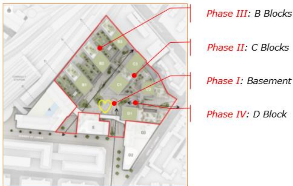
FIGURE 2-8 - CONSTRUCTION PHASING PLAN (INDICATIVE)
